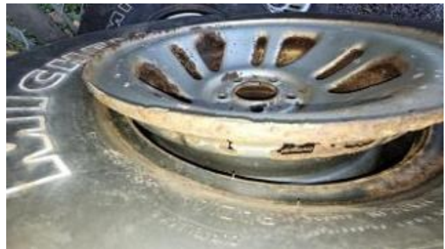
Rust holes in the wheels from sitting
