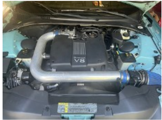
3.9 L V-8 engine making 252 horsepower
