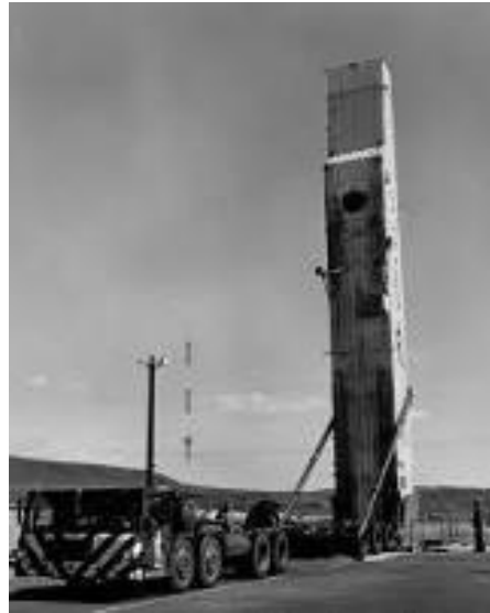
TE in full erect position
