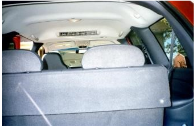
View from cargo door. Note the second air conditioner in the ceiling
