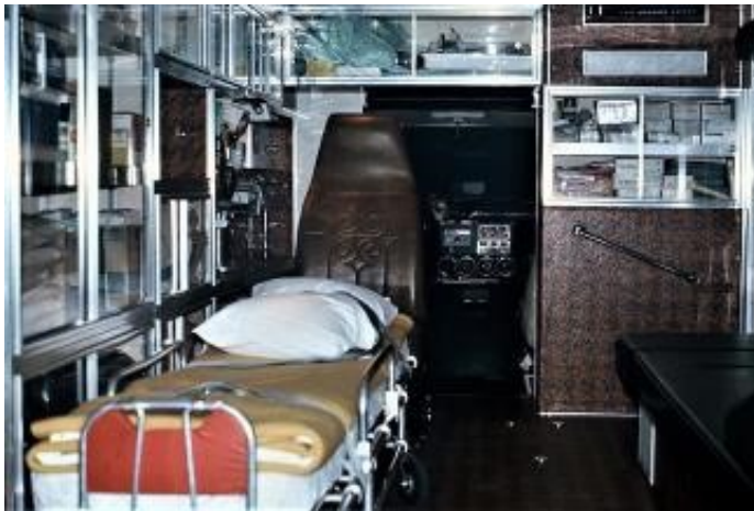
Patient compartment as seen from the rear door. Note the walk-through behind the attendant seat.
