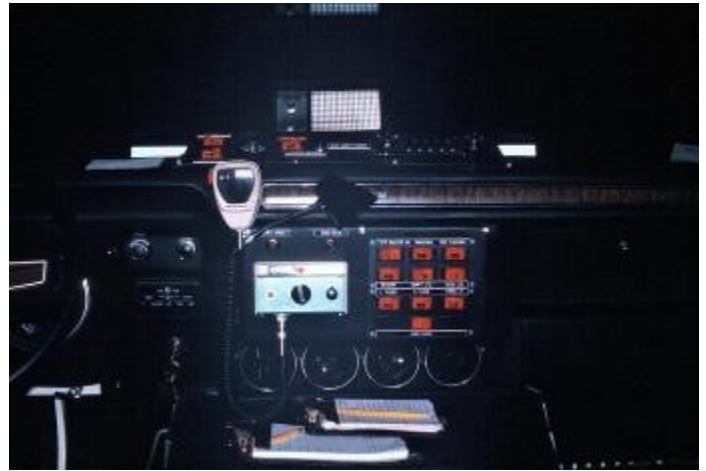
Center console controls for dispatch radio and emergency lights and sirens
