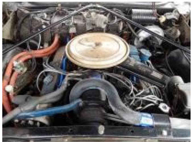
Cadillac 472 cu in engine making 375 hp
