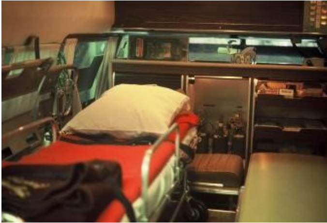
Interior rear view with patient cot and addition of a jump seat at the head of the cot
