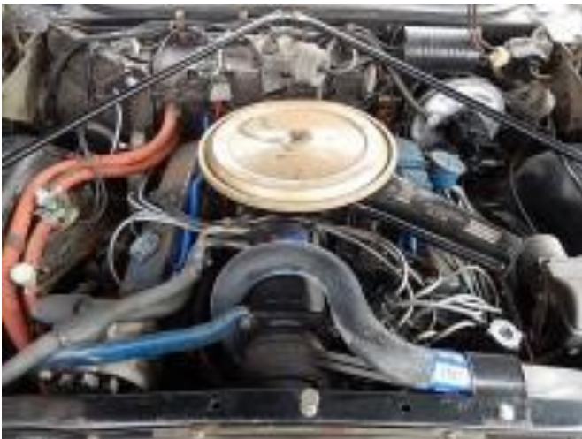
Cadillac 472 cu in engine making 375 hp
