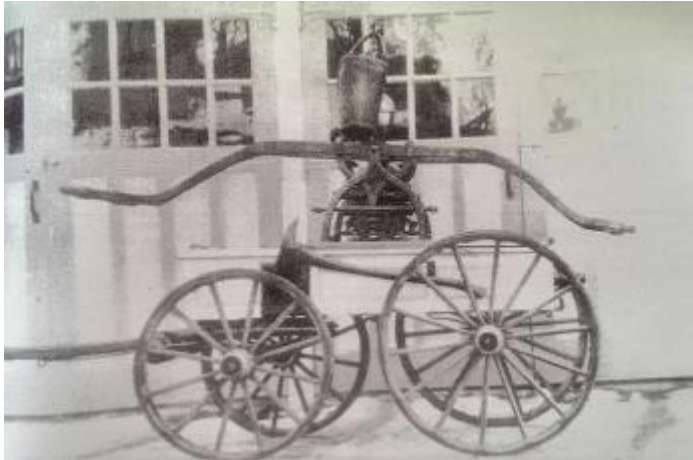
Four person hand pump similar to the one used in Manassas. Output was about 75 GPM
