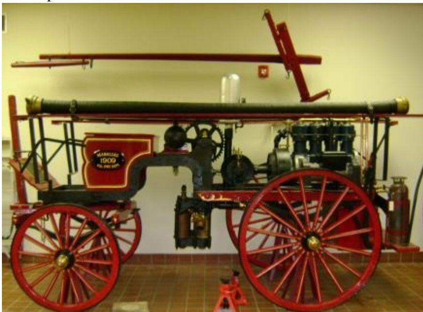
1909 Howe piston pumper with horse harness tongue on the wall above. Short tongue for Model T is attached.
