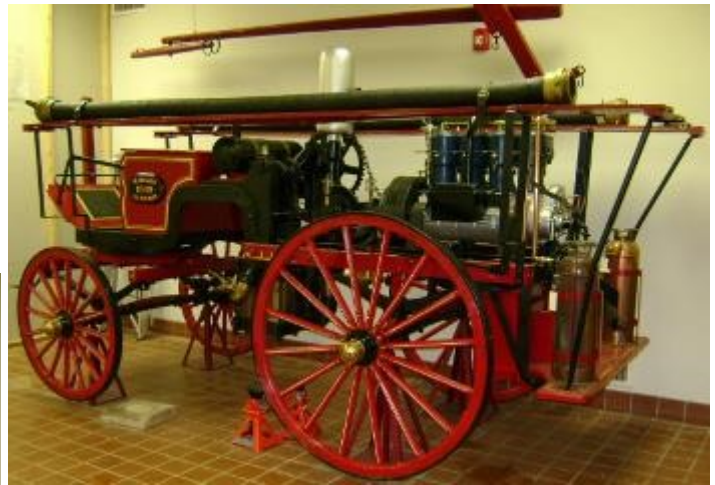
Rear view of the Howe engine, note the prominent engine and silver pressure dome. The rear warning bell can be seen on the right side on the hose frame. Two brass water can fire extinguishers are on the back step.
