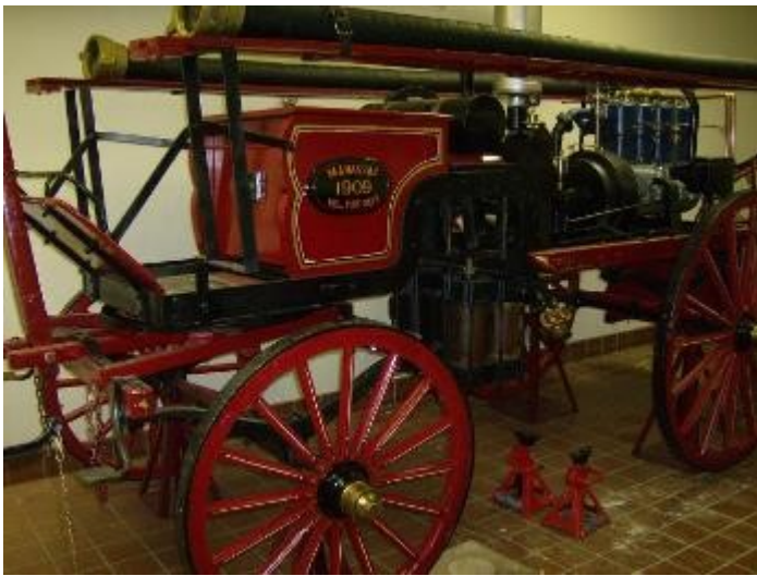
Forward view of the Howe engine, note the brass pump cylinders
