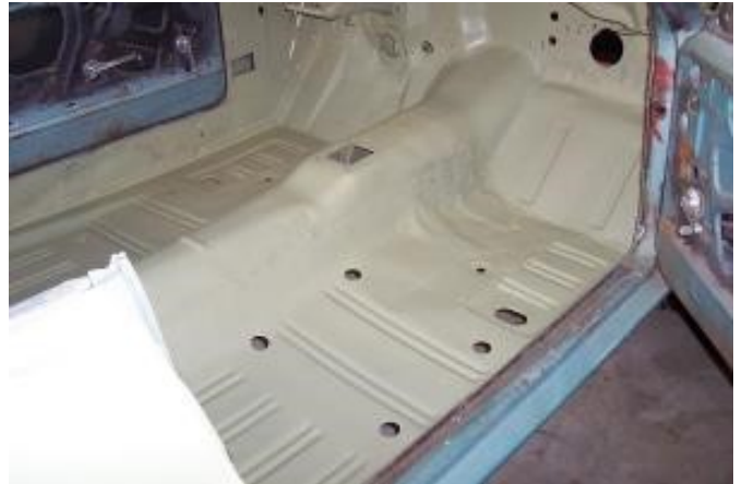
New floor pan installed and primed
