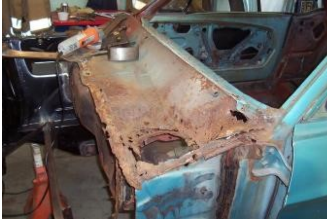
Rusted out cowl, common early Mustang problem
