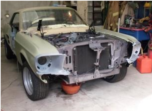
Fenders and rebuilt engine installed
