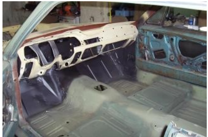
Reproduction dash board installed
