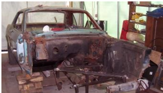
Frame removal using custom alignment jig
