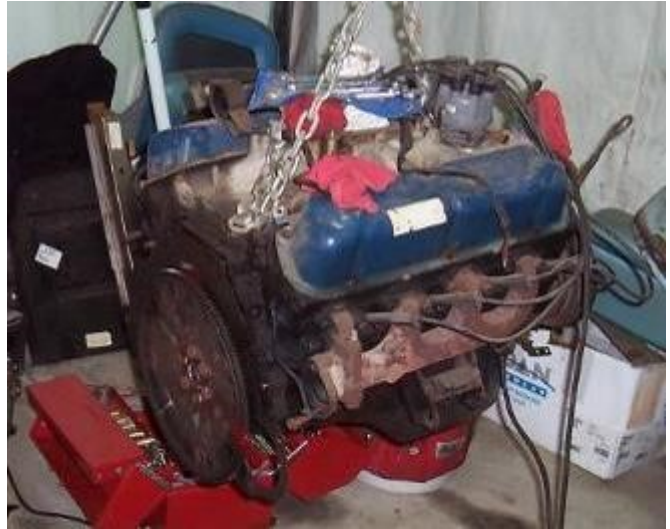
The 302 cu in V-8 after removal
