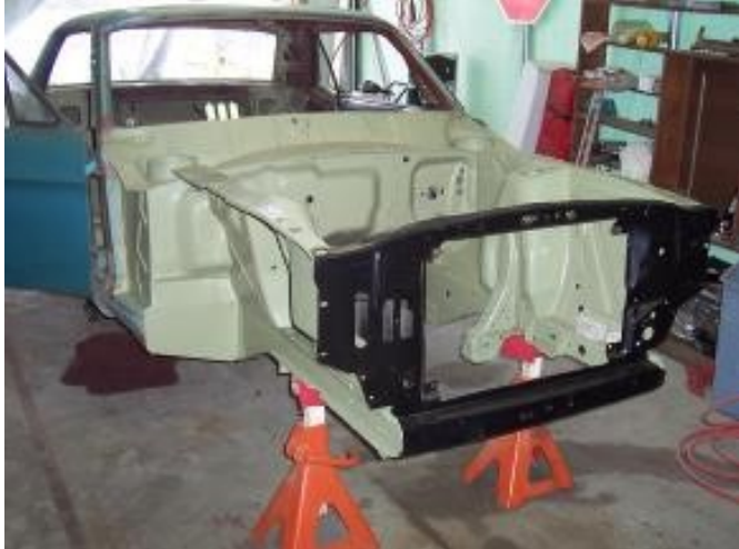
New front frame and sheet metal
