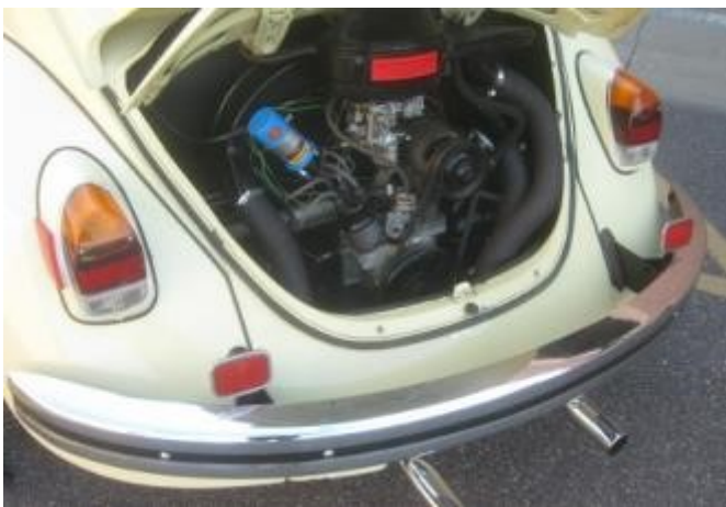
Rear mounted 1600 cc flat four cylinder engine
