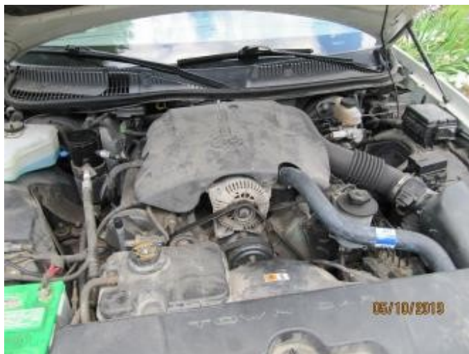
4.6L V-8 engine making 205 hp still dirty
