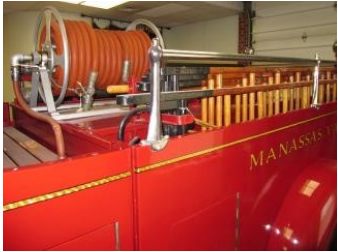
Picture of rear hose reels used on smaller outdoor fires
