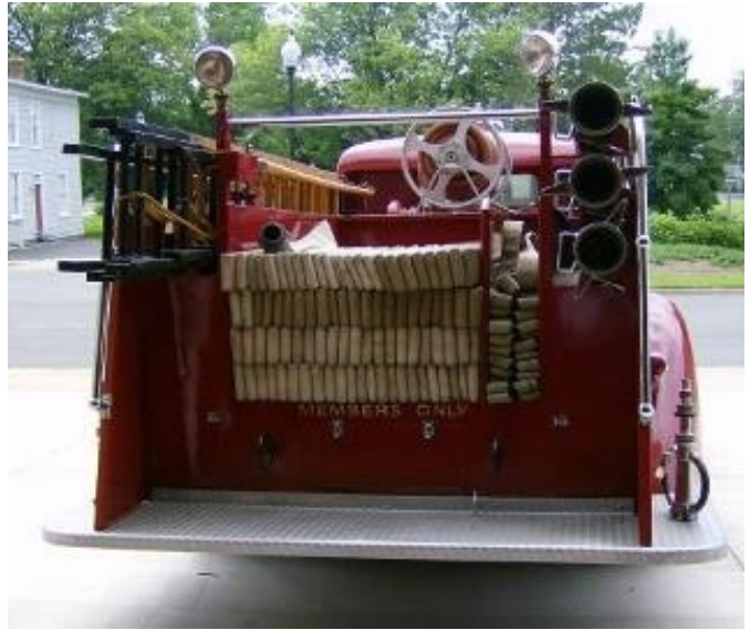
Rear view note hard suction sleeves and ladders held internal to the body
